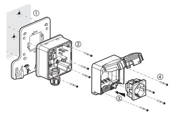
The front part (mechanism cover) is attached to the box using 4 coarse pitch screws.
